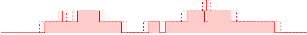
FIG 1. Illustration of the dynamics of the q -PNG. The solid line denotes the height profile at a time t , while the dotted broken line denotes the height functions at a slightly later time t' . Thin vertical lines denote nucleations that took place in the time interval (t, t') .
